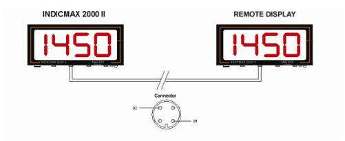
The remote display is not a reader so it can be used only along with the Indicmax 2000 II. It requires an independent power supply and can be installed up to 3000 feet distance by a common pair of wire.
